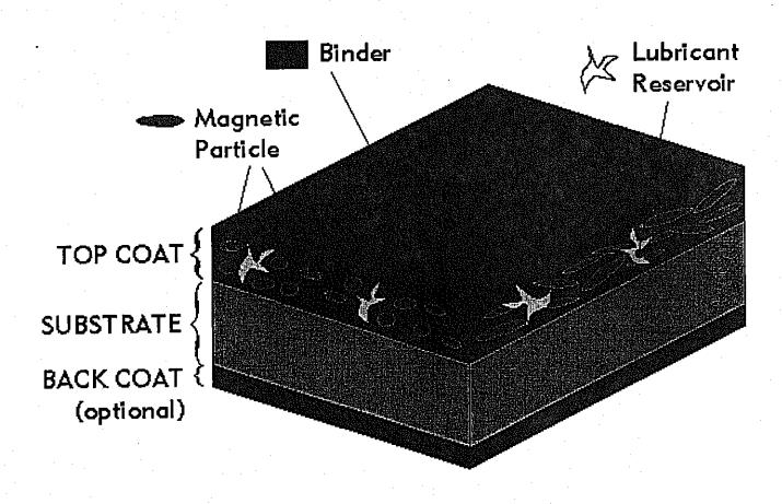
Figure 2. Cross Section of Magnetic Tape
