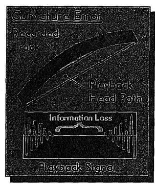
Figure 4. Types of Mistracking for Helical Scan Recording
