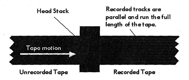
Figure 5. Longitudinal Recording
