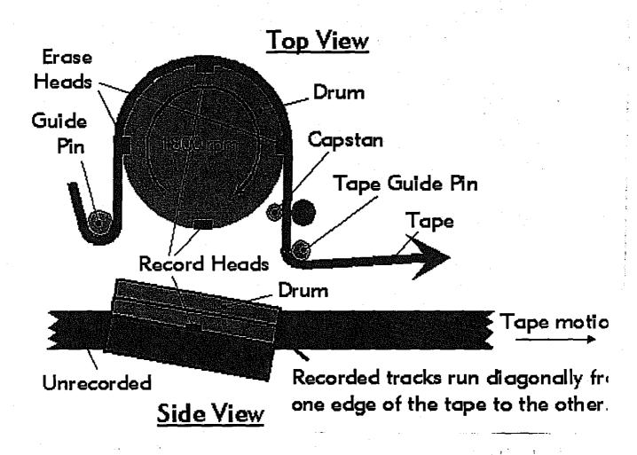
Figure 3. Helical Scan Recording
